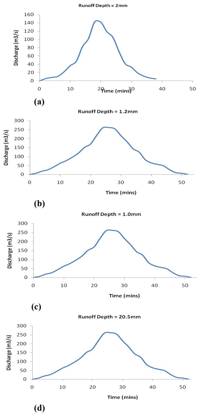
Fig. 6: Hydrographs for the field discharge measurements.
